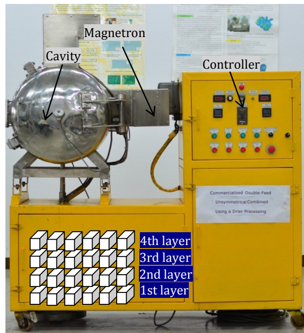
Figure 3 Details of a combined unsymmetrical double-feed microwave and vacuum system. (At the Center of Excellence in Electromagnetic Energy Utilization in Engineering (CEEE). Faculty of Engineering Thammasat University (Rangsit Campus))
